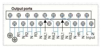
Input Ports L, N: for power connection, L: live wire, N: zero wire, protective ground wire Output R1:Semiconductor relays (SCR), designed for pump speed control, Max. Current: 1A Output R2: Semiconductor relays (SCR), designed for pump speed control, Max. Current: 1A Output R3: Semiconductor relays (SCR), designed for pump speed control, Max. Current: 1A Output R4:Electromagnetic relays, designed for on/off control of pump or 3-ways
