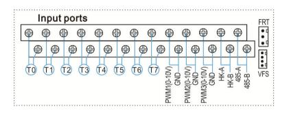
T0~T1: PT1000 temperature sensor, for measuring the temperature of collector
