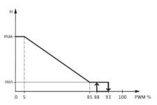
• 0-10: PWM 0 - 10 V signal logic of Speed control
