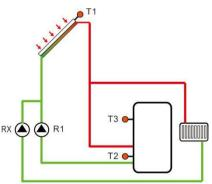
Heat transfer by collector valve logic
