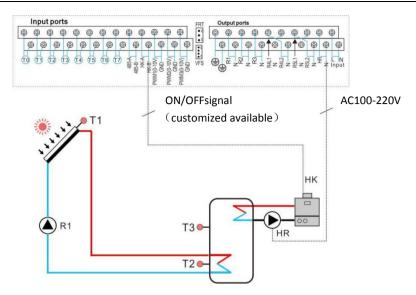
If boiler is selected as back-up heat producer, output HK and HR is controlled by T3 or T2(Optional). When T3 or T2(Optional) is reached to the switch-on temperature of back-up heating function, then back-up heating output HK and HR are triggered, when T3 or T2(Optional) is exceeded the switch-off temperature of back-up heating function, then back-up heating output HK and HR are closed.
