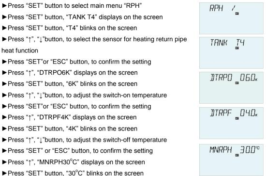
▶ Press "↑", "↓"button, to adjust the minimum temperature of heating return pipe
