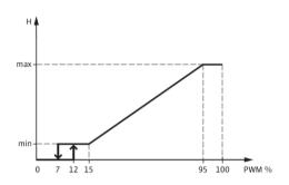
• PHEA: PWM signal logic of heating pump
